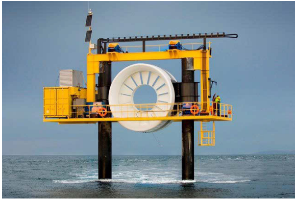
FIGURE 8. Open hydro turbine at EMEC tidal test site [38].
