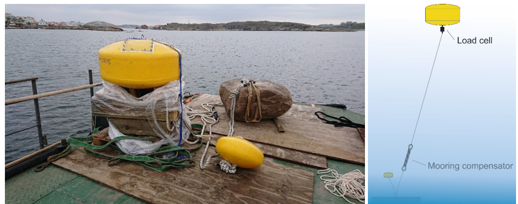
Figure 1. Left picture shows the experimental setup just before deployment. The right figure shows a sketch of the setup. The small buoy at the bottom is used to lift the shackle connecting the line and foundation in order to avoid wear on the line.
