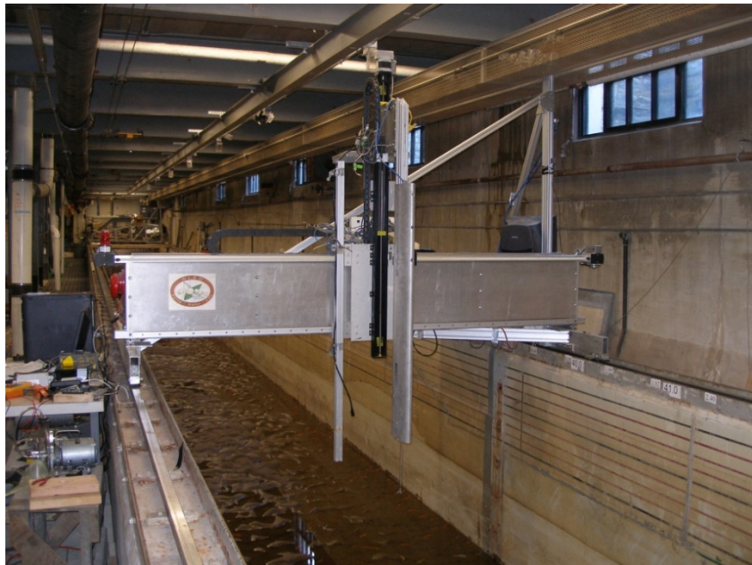
Figure 4b: The SAFL Main Channel DAQ Carriage.
