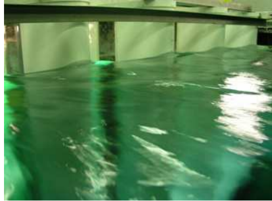
Figure 15: Flow around a 5 tubes network at a flow speed of 1 m/s
