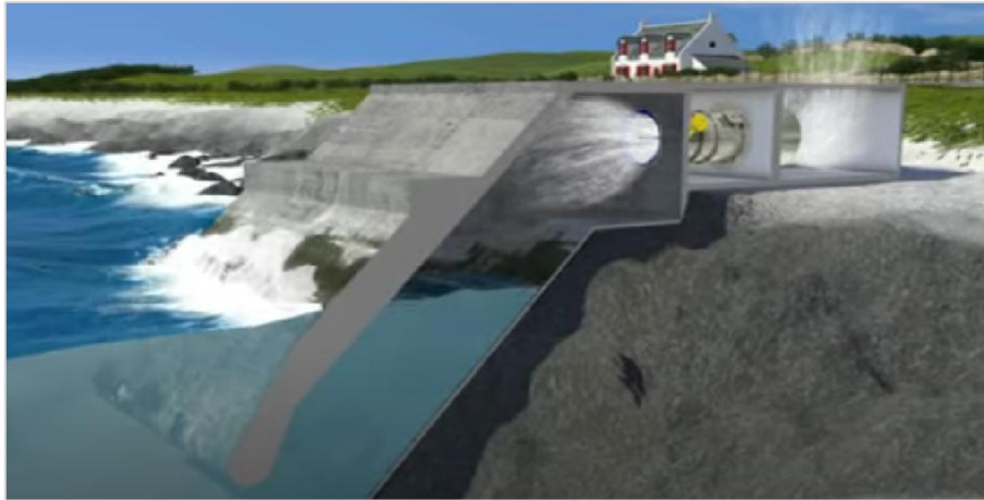
Figure 3. Concept of Oscillating Water Column [50]
