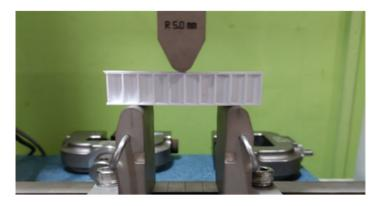
Figure 8. Experimental bending test setup.
