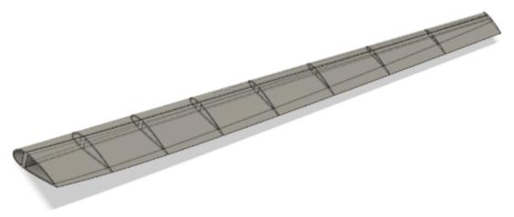
Figure 12. Shell-Spar blade model.
