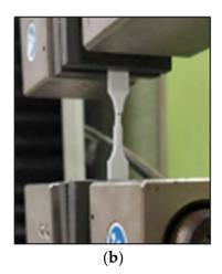
Figure 5. Tensile test experiment (a) before test, (b) failure after test.
