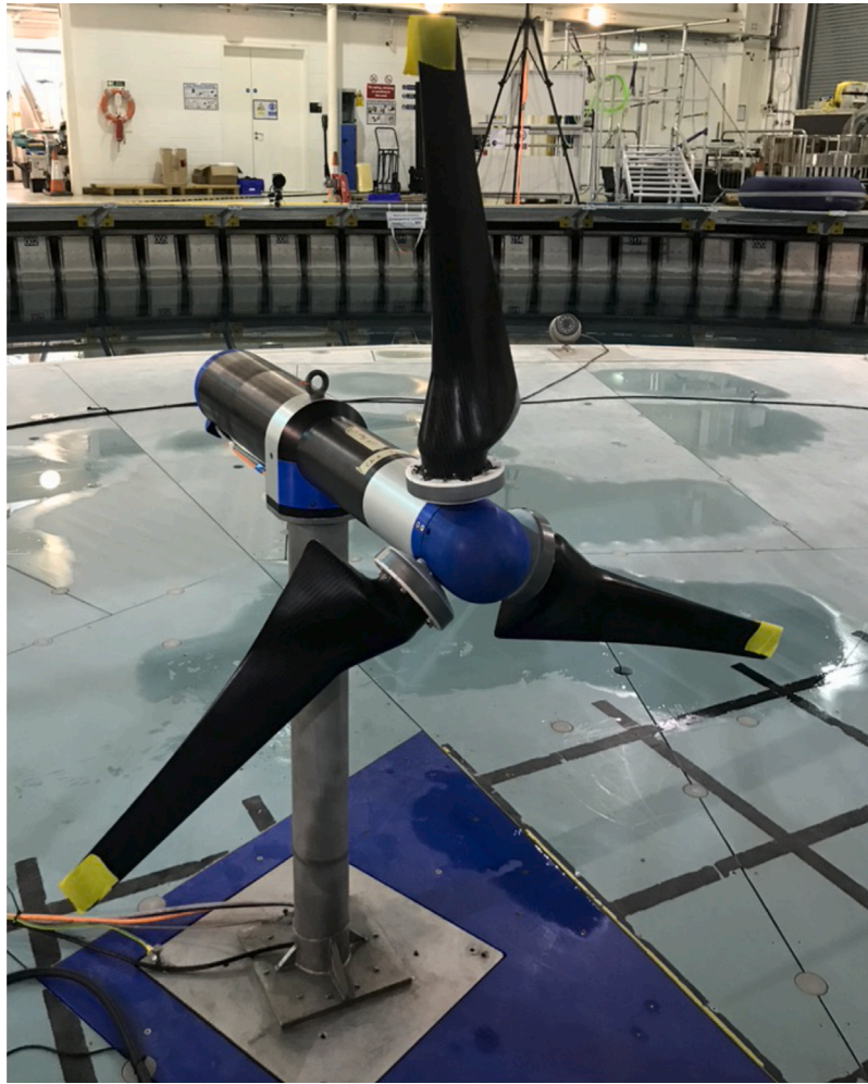
Fig. 5. The model-scale tidal turbine installed on the raised floor of FloWave (the yellow tape at the tip of the blades is removed during testing).
