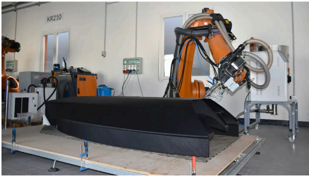
Fig. 10. LFAM printed dinghy sailboat made of thermoplastic. Image courtesy of Caracol.
