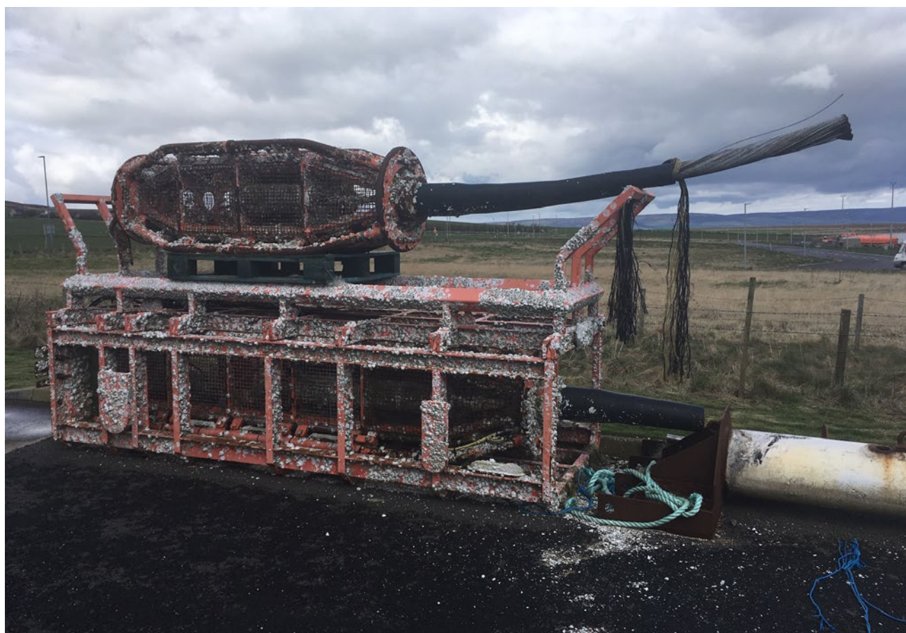
Figure 15. Two electrical connection hubs, one on top of the other, used at the wave test site of EMEC (Orkney, Scotland) and expanded view of barnacle colonization after three years at sea.
