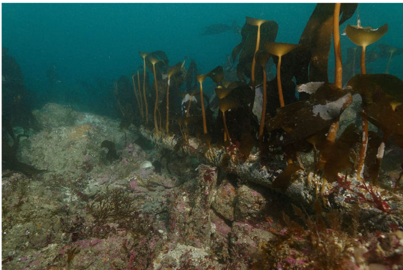
Figure 13. Colonization of a cable deployed in a rocky environment of the SABELLA tidal test-site (France). A high density of kelp ( Laminaria hyperborea ) was observed on the naked cable.
