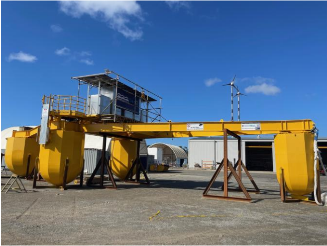
Fig 4. M4 WED during assembly. Bow and stern arms connected to floaters with PTO and control cabinet installed.
