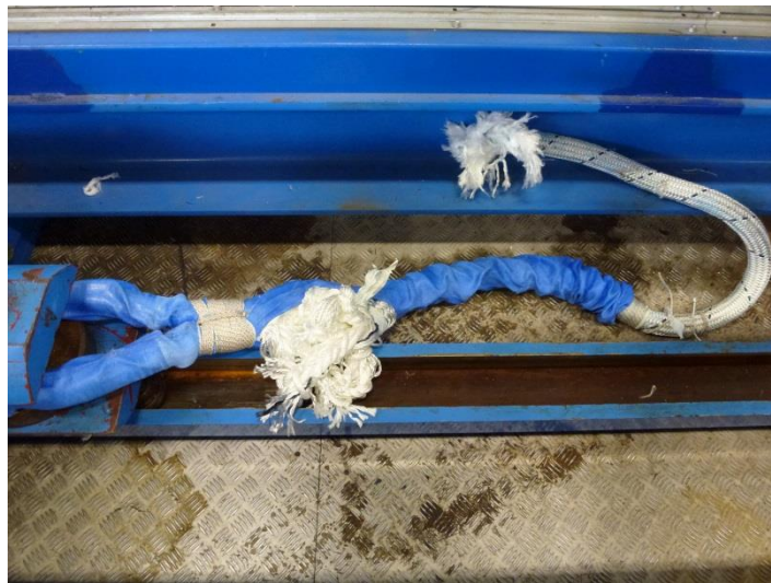
Figure 4: The inevitable result of a load-to-failure test of a new nylon mooring rope sample (test conducted at IFREMER as part of the MERiFIC WP3.5 study)
