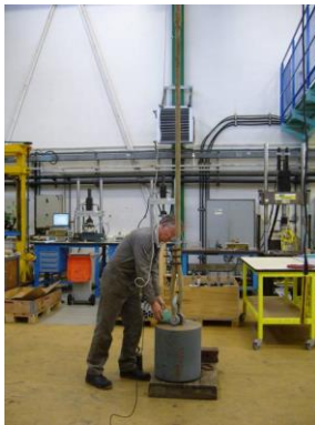
Figure 9: Axial natural period tests conducted at IFREMER as part of the MERiFIC WP3.5 study; (left) experimental set-up, (right) filtered load cell response after impulse excitation
