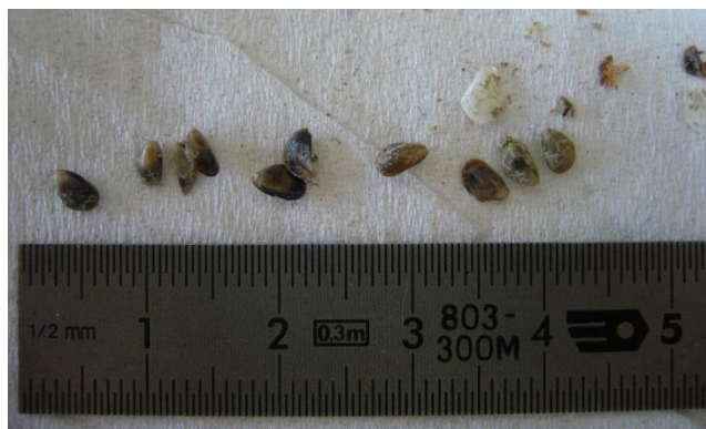
Figure 14: Juvenile mussel shells found on the inside of the projective jacket of the aged rope sample used for the MERiFIC WP3.5 study
