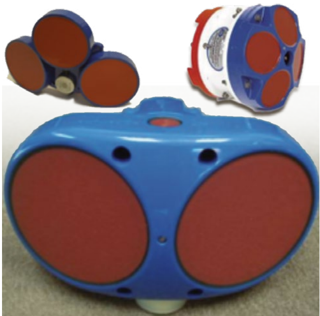
Figure 8. Different types of ADCP beam configurations (RDI 2011)
