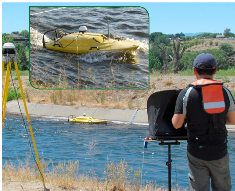
Figure 4. The remote control survey boat with real-time kinematic GPS correction.
