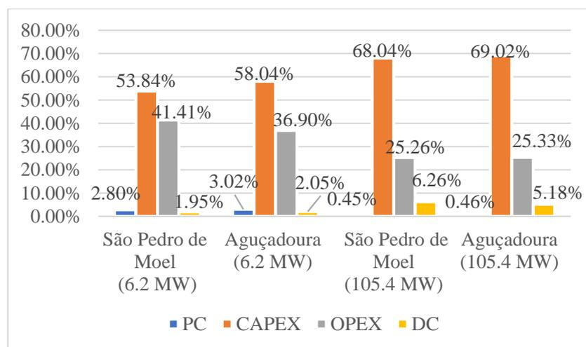
Figure 7. Percentage of the cost center towards total cost of Poseidon technology (Note: Figure does not show discounted cost for the 100-unit Pelamis installation).
