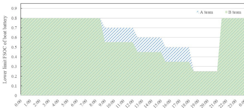
Fig. 7. The daily peak period control and phased deep discharge schedule for lower limits of boat batteries.
