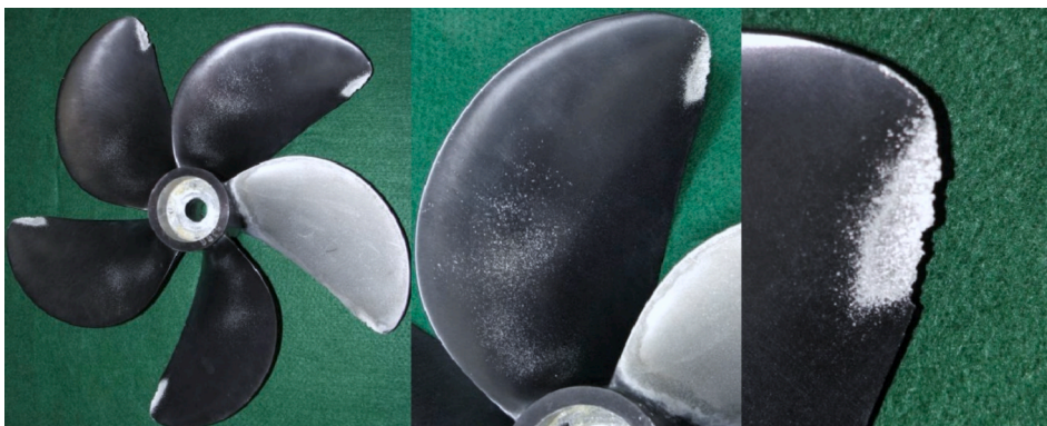
Fig. 16. Cavitation-induced erosion on the trailing edge of a blade [118].
