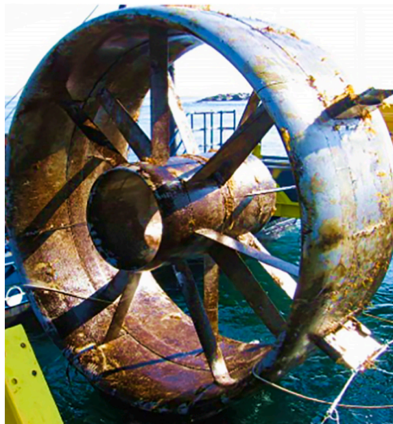
Fig. 11. Fouled tidal turbine six months after commissioning [7].
