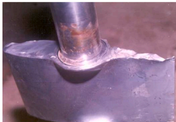
Fig. 19. Erosion on hydro turbine metal components caused by impact-induced damage [113].
