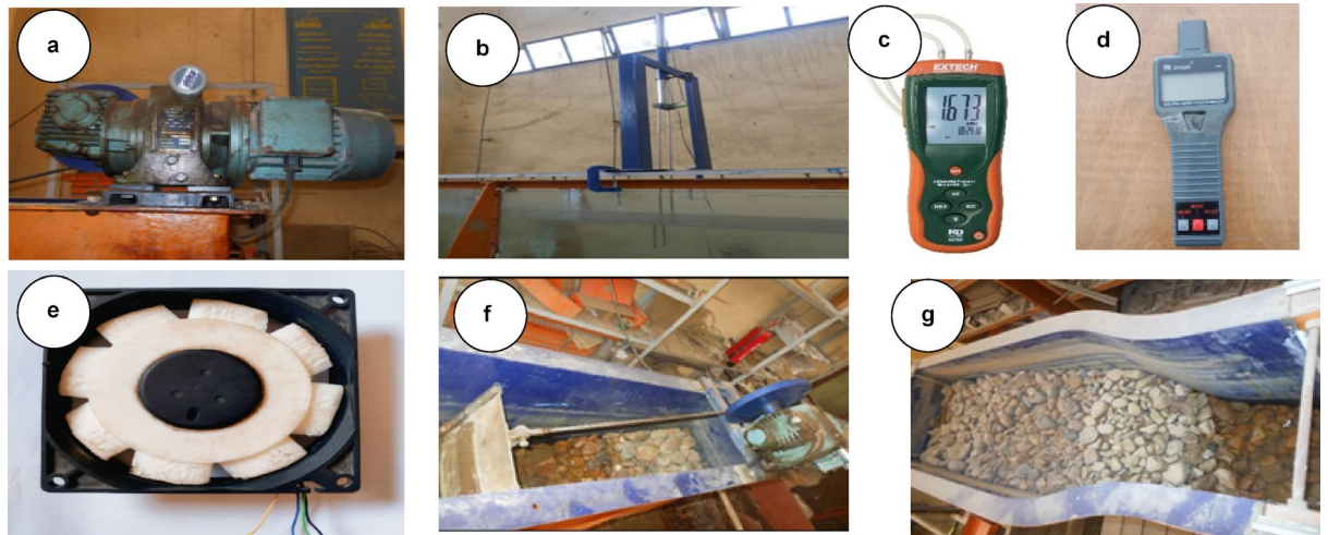
Fig. 2. Instrumentation setup onboard the FBW-WEC models: (a) Wave maker, (b) Wave probe, (c) Pressure gauge, (d) Tachometer, (e) PTO and voltmeters, (f) First absorber, and (g) End absorber.
