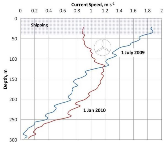
Figure 1: Current speed as a function of depth in the Florida Current 16 km offshore Dania Beach. The stippled area at the top denotes a shipping-lane depth zone, and the symbol represents (to scale) a 40-m diameter system deployed at 70 m. Note that the sign of the vertical shear in this layer is different for the two profiles.
