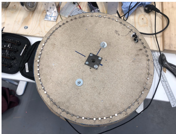
(a) Unattached wheel showing the rim layout with 72 alternating magnets.
