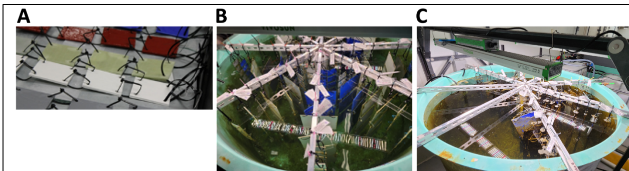
Figure 9 | Coupons prepared and suspended in biofouling tanks. A. Depiction of the daisy chain hanging style where 3 in 2 coupons are shown zip-tied to each other. B. E-Wave biofouling tank 1 month after all coupon samples were submerged. C. E-Wave biofouling tank photo taken after 6 months (note that 3- and 6-month time point coupons had been pulled for processing).
