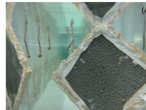
Metal – Carbon Fiber Composite Interconnects in Seawater
