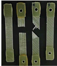
Salt Water Effects on Composite Performance Testing
