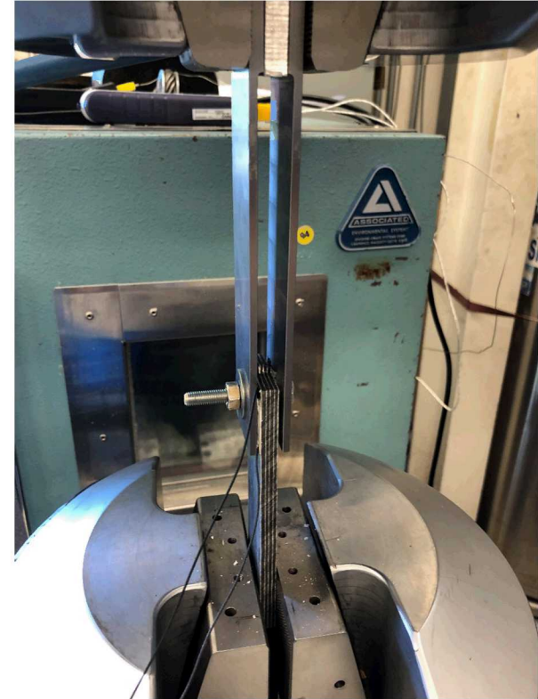
Test procedure: ASTM D5961: Standard Test Method for Bearing Response of Polymer Matrix Composite Laminates
