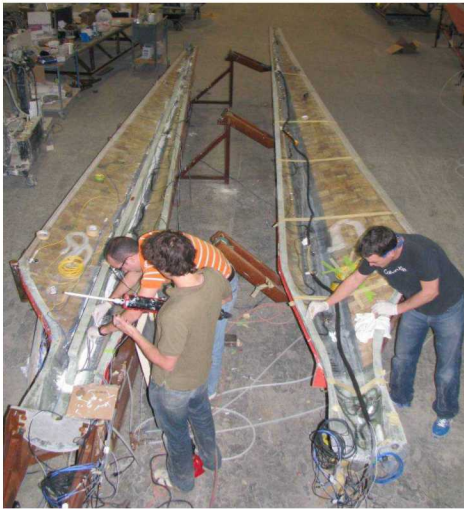
Fiber optic strain sensor on wind blades
