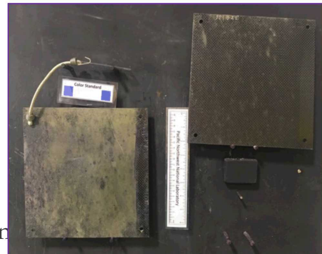
Bad (L) and good (R) performance on carbon fiber, 6 months
