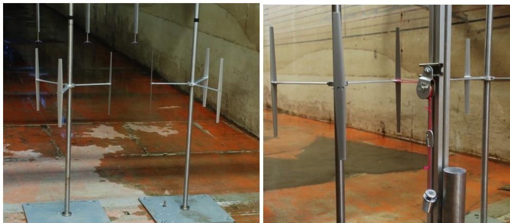
Figure 3: Photos of the RM2 dual-rotor model in the SAFL Main Channel (left) and during torque sensor calibration (right) performed by applying known forces to the rotor and torque sensor.
