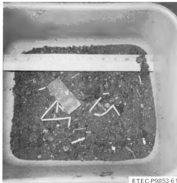
Figure 5-47. Contamination from Ammonia Loop
