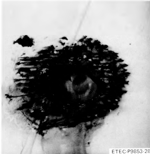
Figure 5-15. Ultrasonic Flowmeter Window, Portside
