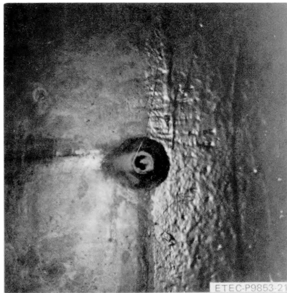
Figure 5-8. Inlet Waterbox Static Pressure Tap
