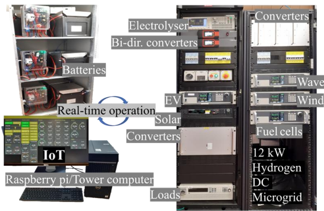
Fig. 4: Bench-scale experimental set up at Griffith University
