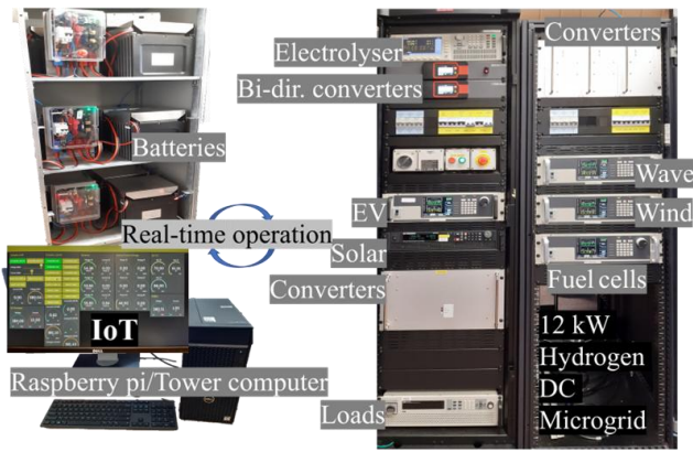
Fig. 4: Bench-scale experimental set up at Griffith University
