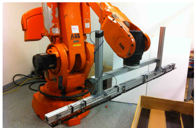
Figure 4: An industrial robot lifting a G3 UU WEC stator plate using a prototype stacking tool currently under development
