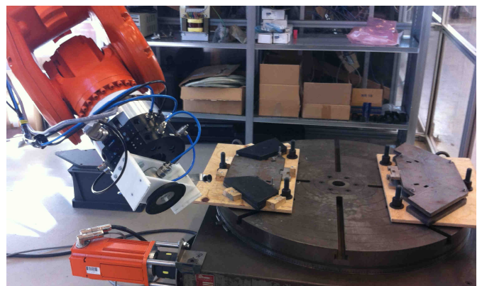
Figure 8: An experiment with an industrial robot assembling ferrite magnets on G3 UU WEC pole sheets placed on a rotary table
