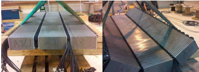
Figure 5: A cable wound G3 UU WEC stator section, (Left) before being folded and (Right) after being folded
