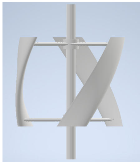
Figure 2. Physical structure of the Gorlov turbine.
