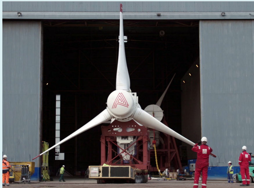
The AR1500 tidal turbine (Source: SAE Renewables)
