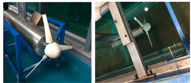
Fig. 4. Tidal Energy Converter and Experimental Procedure.
