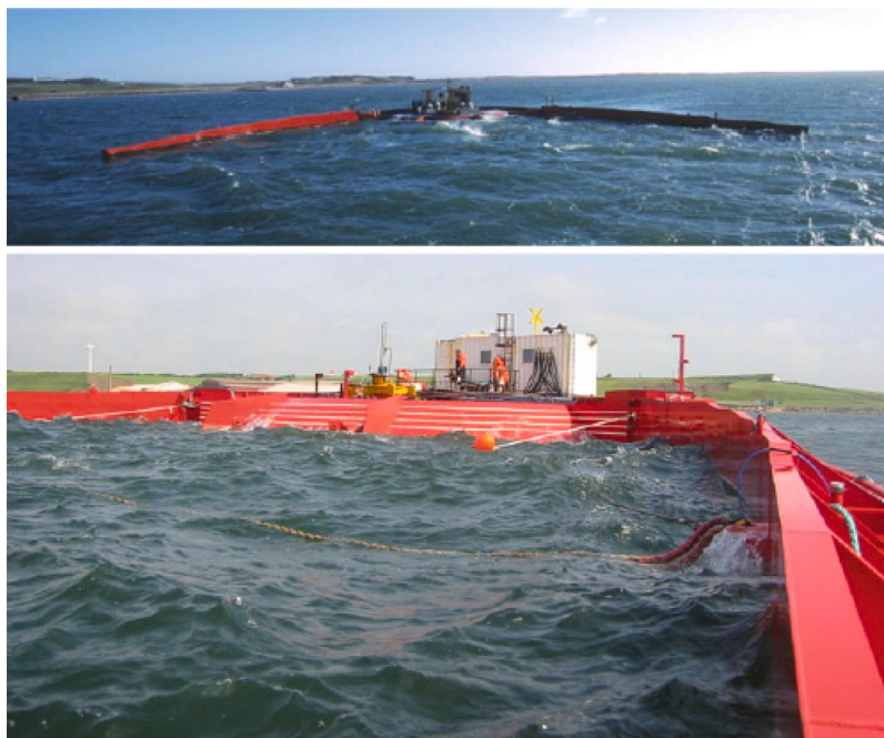
Fig. 9. 1:4.5 scale of the Wave Dragon converter. Source: From [23].
