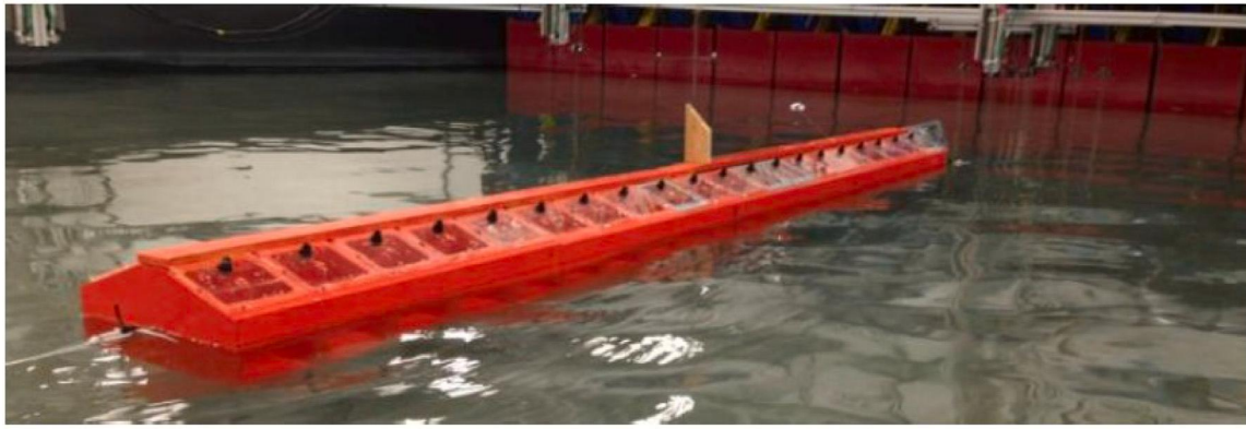
Fig. 7. Experimental model scale of the KNSwing device. Source: From [35].
