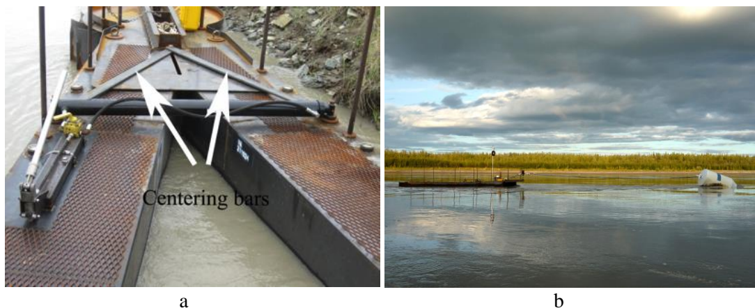
Figure 9. RDDP centering bars, hydraulic ram, and pump systems (a), and RDDP tethered to the mooring buoy (b).
