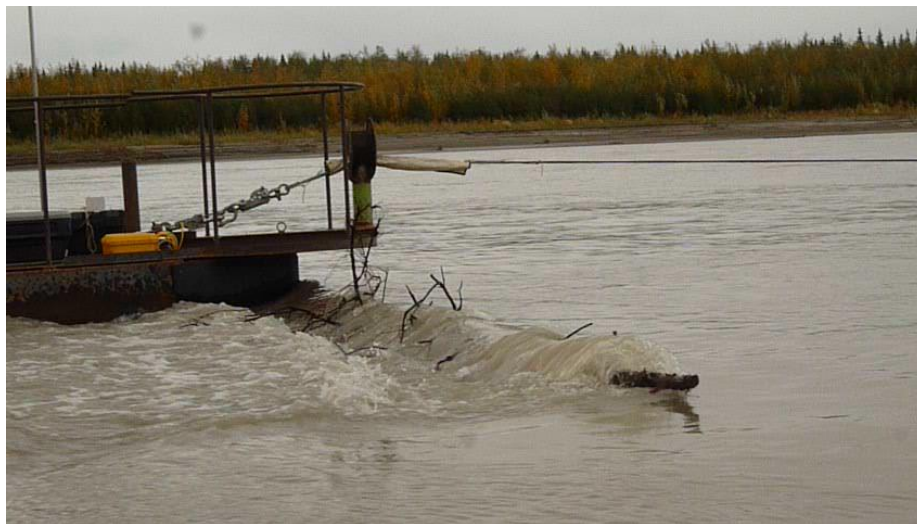
Figure 20. Debris object impinged against the sharp-angled RDDP front end, 62-degree angle.
