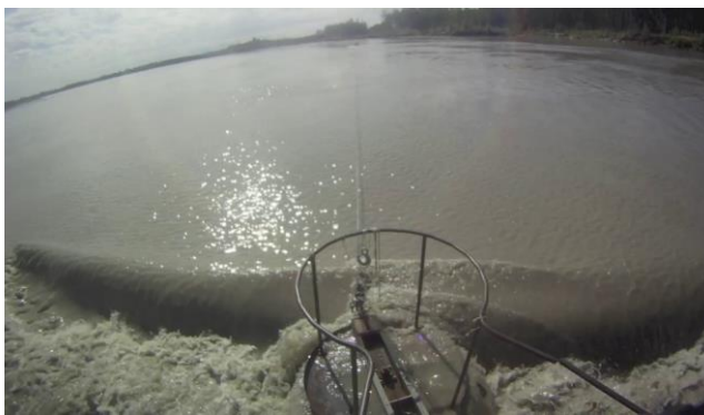
Figure 19. Debris object torque balanced on the RDDP's debris sweep with hinged vanes.
