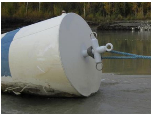
Figure 11. Mooring buoy (1.2 m diameter by 1.9 m length cylinder with a 1.9 m length conical section on the anchor chain end) with RDDP mooring line on its bitt.
