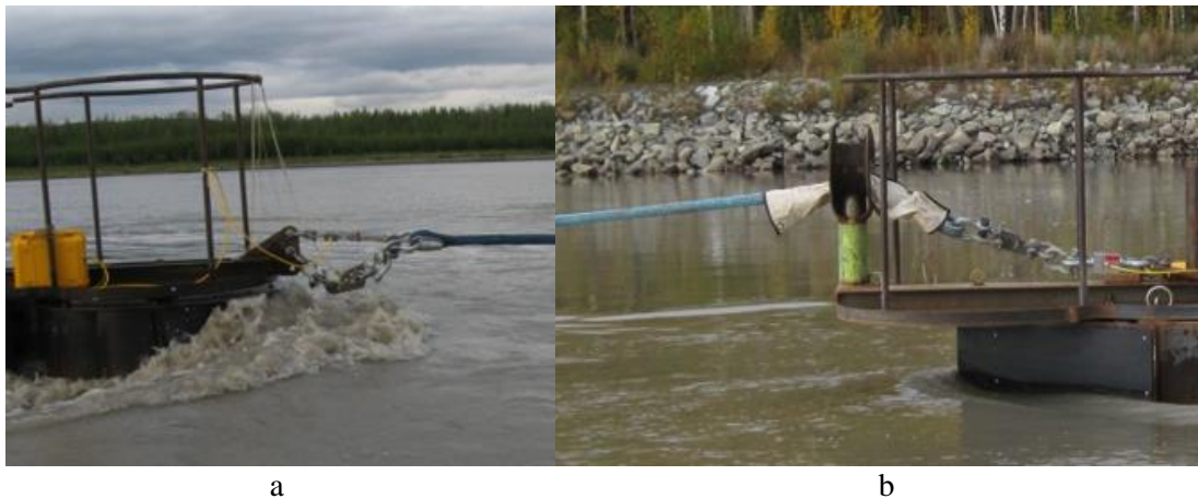
Figure 10. RDDP original mooring attachment system with hinged-vane debris sweep (a) and modified attachment system with sharp-angle front end (b).
