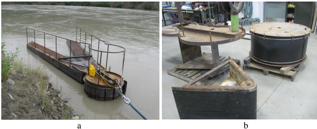
Figure E1. RDDP in its closed position showing the debris sweep with hinged vanes (a) and the RDDP front-end mount shown separately from the plastic-covered angled front end and the plastic-covered debris sweep cylinder (b).
