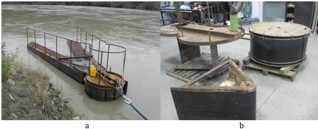
Figure 8. RDDP in its closed position showing the debris sweep with hinged vanes (a), and the RDDP front-end mounts shown separately from the plastic-covered V-“nose” 62-degree angled front end and the plastic-covered debris sweep cylinder (b).
