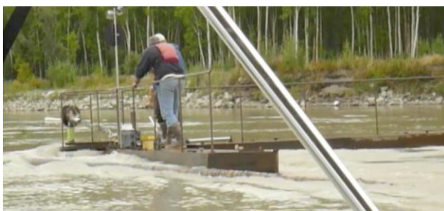
Figure 26. Debris object pinned to the RDDP pontoon, with a pontoon opening angle of greater than 75 degrees.
