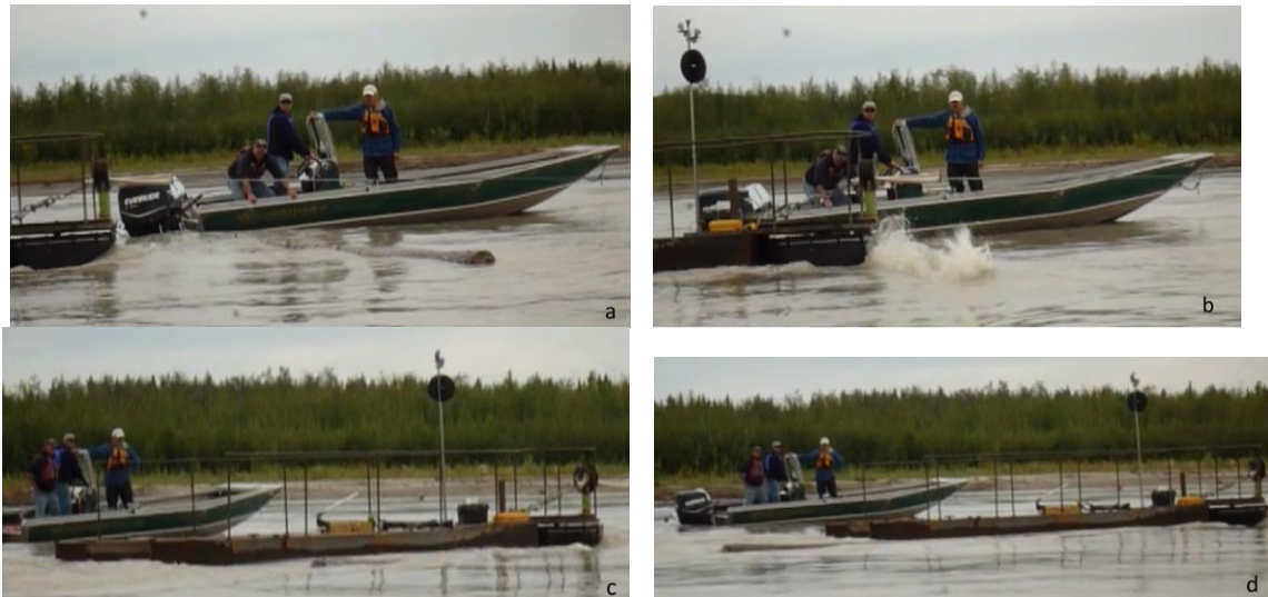
Figure 13. Direct debris impact test of the RDDP using a log perpendicular to the current flow direction. Debris object just before impact (a), on impact (b), sliding off the debris sweep (c), and clearing the RDDP (d).
