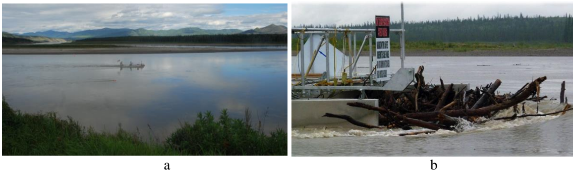
Figure 1. New Energy 25 kW hydrokinetic power turbine on the Yukon River at Eagle, Alaska, August 2010 (photo credit: J. Johnson) (a) and debris accumulation in front of the turbine barge (photo credit: Alaska Power & Telephone) (Johnson and Pride 2010; Johnson et al. 2013).
