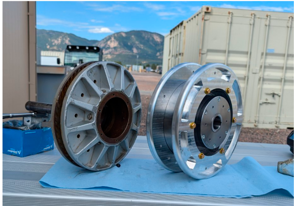
Figure 5. HERO WEC wire rope winch (left) and spiral initiating winch used for belt testing (right). Image Credit: Scott Jenne, NREL.
