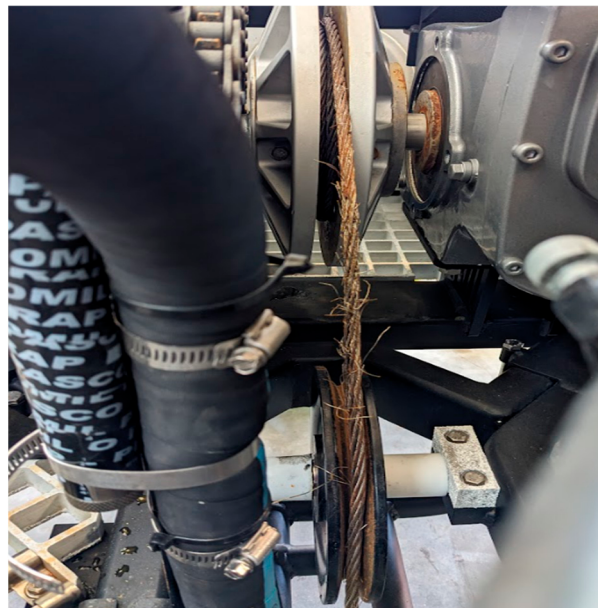
Figure 2. Example of wire rope fatigue and abrasion damage observed after the 2024 hydraulic configuration deployment. Image credit: Patterson Taylor, CSI.
