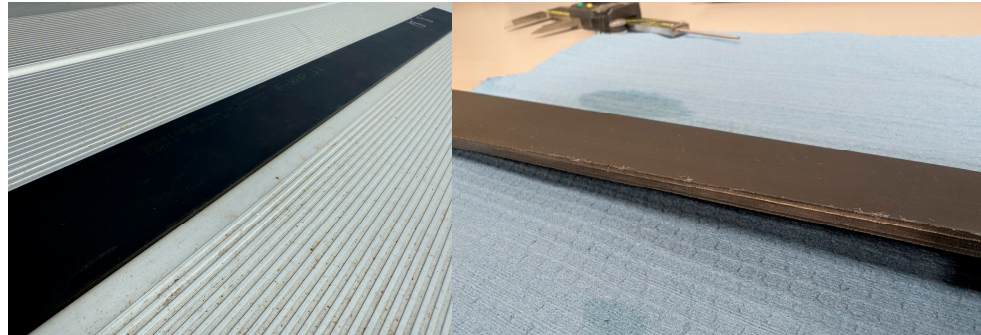
Figure 13. Left: edge of belt as received from Continental. Right: Corner abrasion observed on belt after dynamic testing. Image Credit: Justin Panzarella, NREL.
