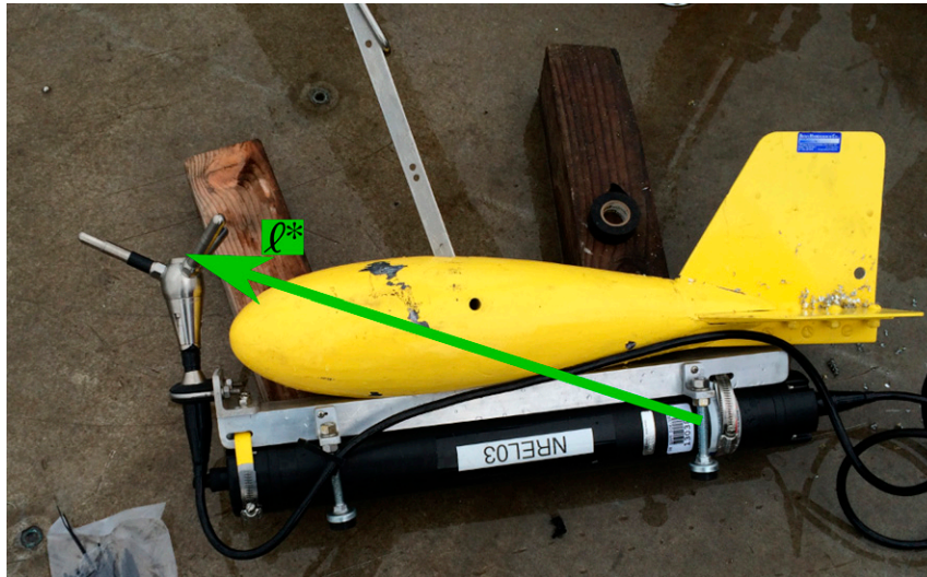
FIG. 5. The turbulence platform showing details of the ADV head and pressure case configuration. The green arrow indicates the vector from the IMU to the ADV head. The head cable was taped out of the way beneath the sounding-weight tail fins shortly after this photograph was taken.
