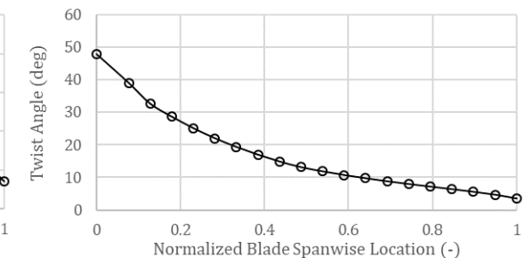
Blade section chord length and twist angle along the spanwise location of the blade
