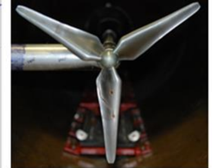
Illustration of the model rotor and dynamometer installed in the GTWT test section, and a photograph of the installed rotor (Fontaine et al., 2020)
