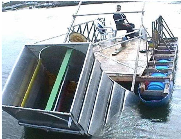
Fig.9. Ducted turbine mounted on motorised barge, tilted partly out of the water to show construction.
