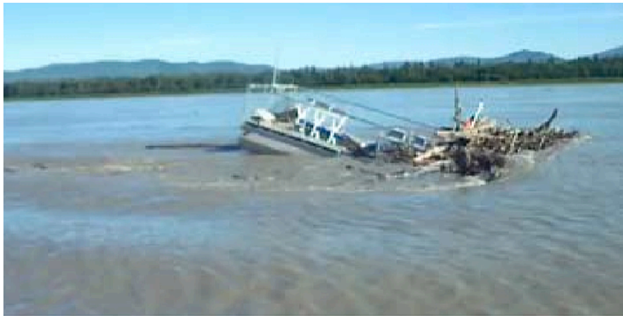
Fig. 19. Debris accumulation on a pontoon-mounted HKT in Alaska (after Tyler, 2011).
