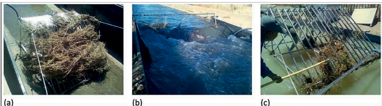
Fig. 20. Debris blocking a pair of Smart Hydro turbines in South Africa (Niebuhr et al., 2021).
