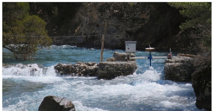
Fig. 4. New Energy Corporation's 5 kW turbine on left, floating, on right, fixed mounting in partially blocked river (from https://www.newenergycorp.ca ).
