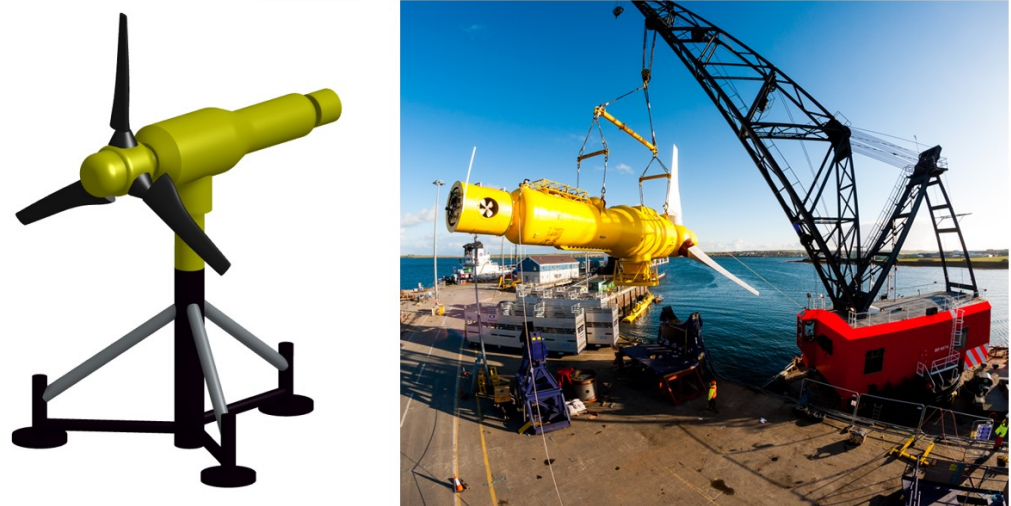
Figure 1. The CAD model of the 1 MW DeepGen-IV tidal turbine (left) and the turbine being deployed from Hatson Quay, Kirkwall, Orkney (right).
