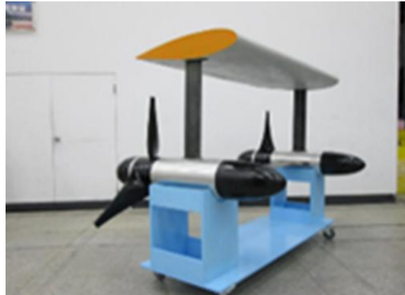
Figure 1 800 W FKT prototype.
