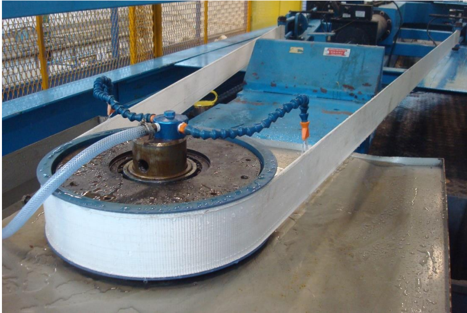
Figure 2.4: Experimental set up with sheave and belt mounted to the test machine.
