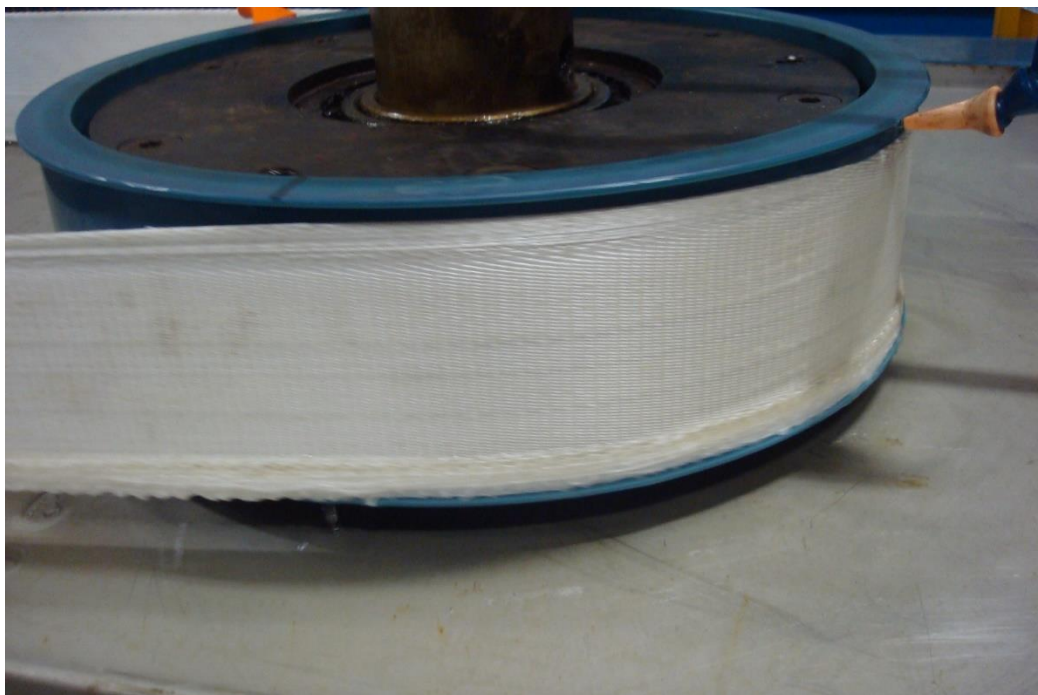
Figure 2.10: Significant visible damage to the bottom edge of the belt noted after 6 days of testing.
