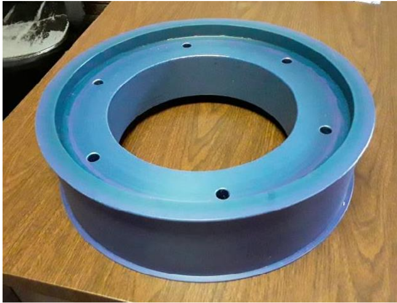
Figure 2.2: Custom pulley sheave machined from Nylon MD Oil-Filled.
