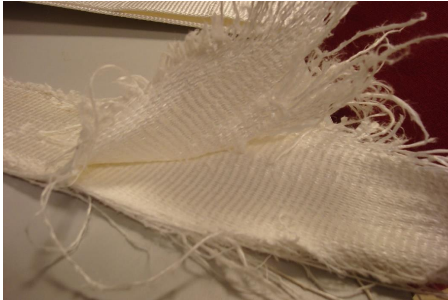
Figure 2.17: Delamination of belt suggesting a layered cross-section construction.
