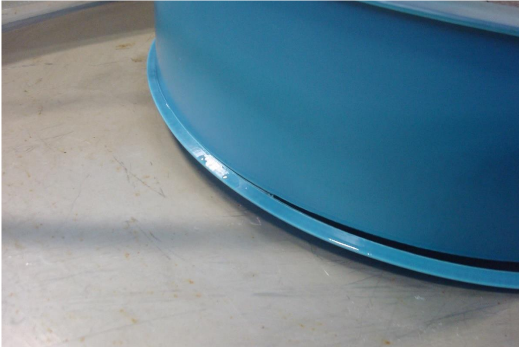
Figure 2.11: Sheave with partial lower flange failure.
