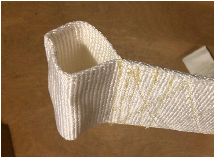
Figure 2.1: HMPE belt construction showing end loop termination.
