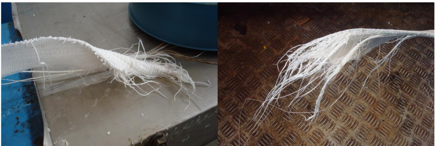
Figure 2.16: Belt after complete failure.
