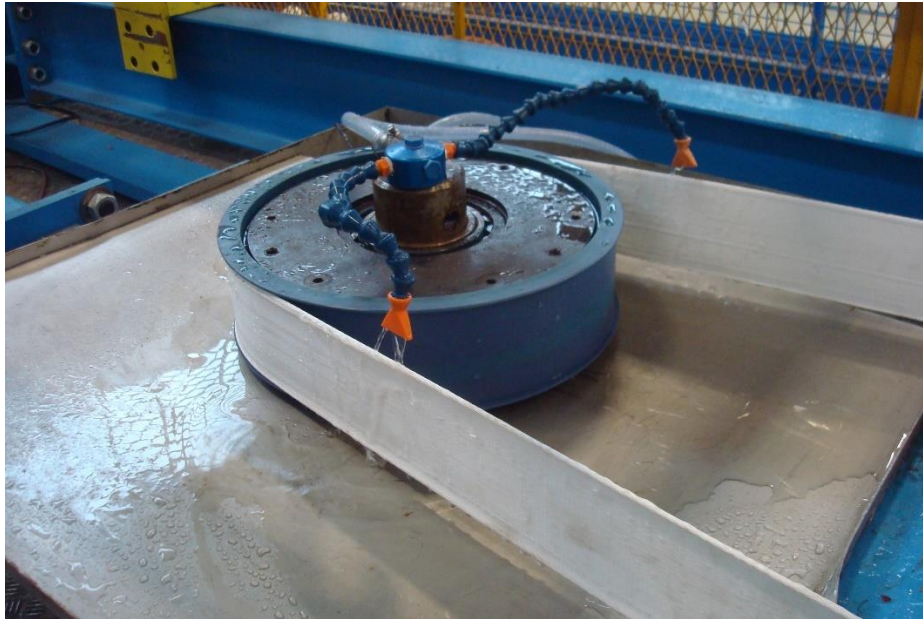
Figure 2.7: Belt showing slight folds at end due to not fitting well inside of the sheave width.
