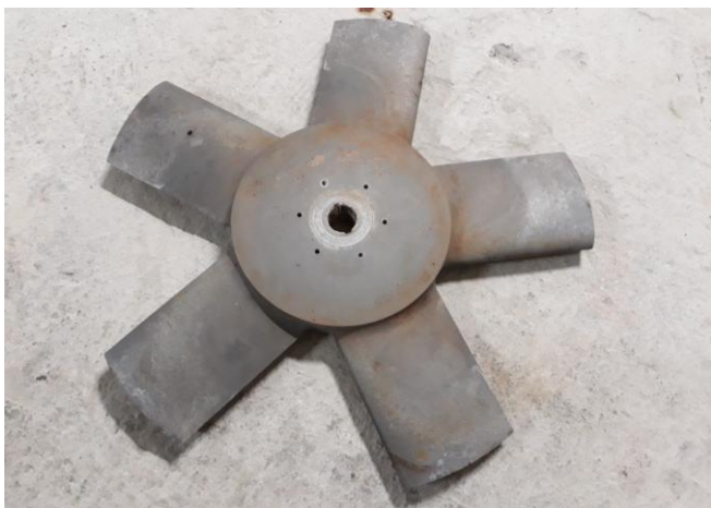
Figure 3: A Wells turbine after five years of operation.
