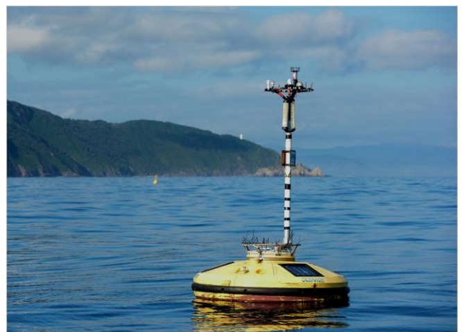
Figure 5: The metocean buoy provides wave and wind parameters in hourly basis
