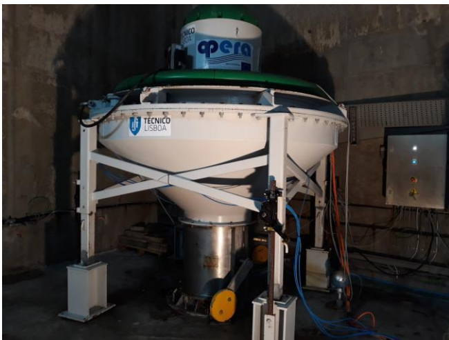
Figure 6: The bi-radial turbine during a test in Mutriku OWC Test Site
