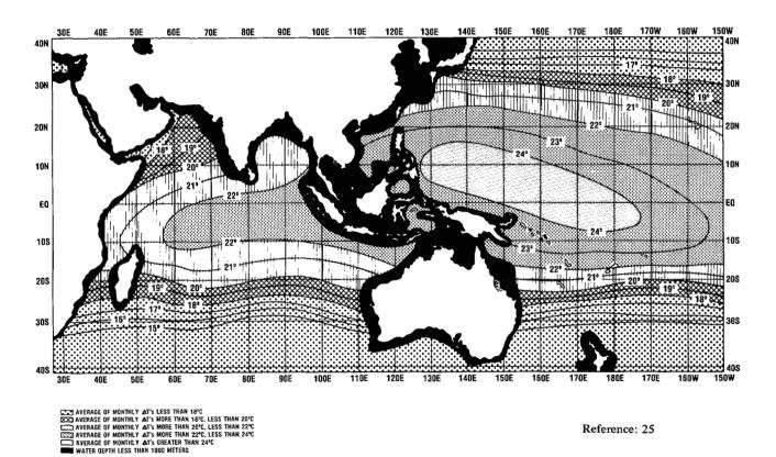
Figure 1. △T(°C) Between Surface and 1000 Meter Depth
