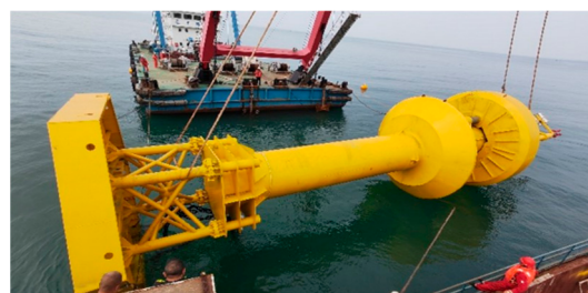
Figure 6. The experimental setup of the SDU-III WEC during sea trials.
