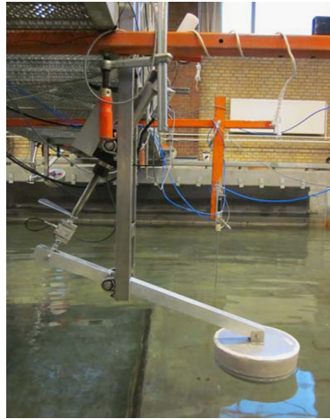
Figure 1.4: The 1:20 scaled Wavestar-like device (Zurkinden et al., 2014) built in Aalborg University.
