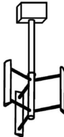
Figure 6 - Cross flow turbines (H-Darrieus Rotor).
