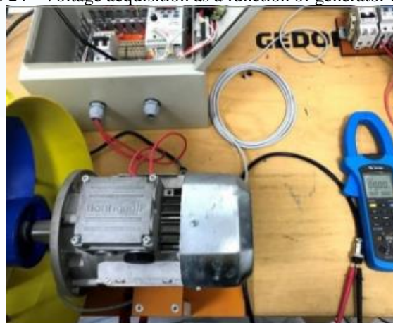
Figure 24 - Voltage acquisition as a function of generator rotation.
