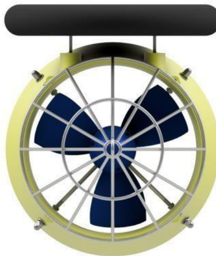
Figure 12 - Hydrokinetic generator concept.
