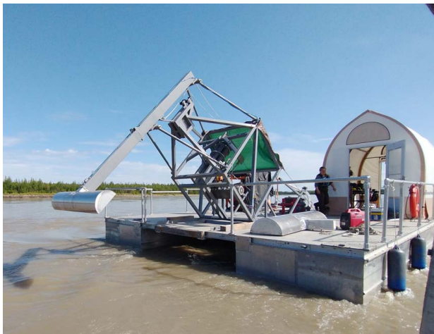
Fig. 5 Water Horse prototype in the “retrieved” position on TRTS research barge
