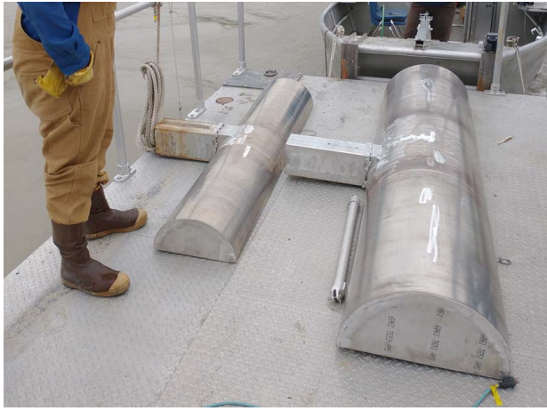
Fig. 7 Small (left) and Large (right) bluff bodies on deck of TRTS research barge between test deployments
