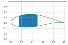
**Figure 5:** The box reinforced in blue for section at r=80mm
