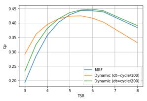
Figure 4: Comparison between MRF and Dynamic method
