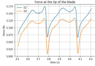
Figure 9: Force at the tip of the blade (in N).
