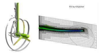
**Figure 12:** Instant view of the simulation showing the isovalue of the Q criterion.
