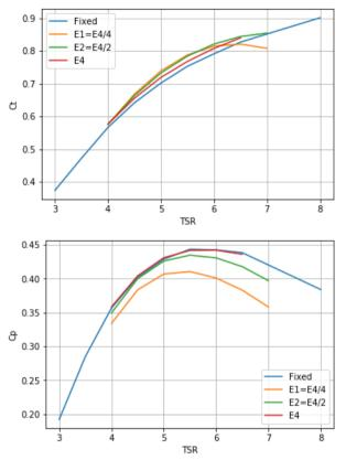
Figure 6: Performance curves for different structural properties.
