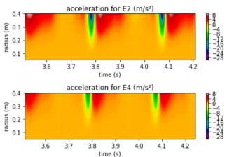
**Figure 11:** Acceleration of each structural node of the blade according to time (in m/s²).
