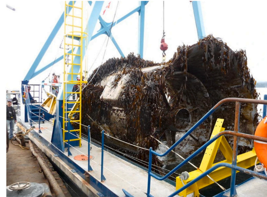
(d) Ducted axial-flow tidal current turbine after three years of deployment in the Race Rocks Ecological Reserve in British Columbia, Canada (66).
