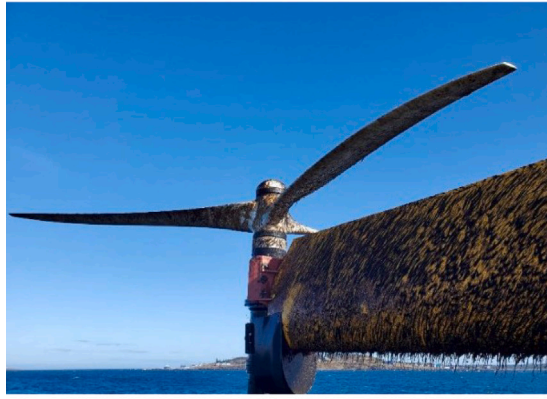
(a) Fouled condition of the SCHOTTEL Instream Turbine (SIT), achieved by keeping the rotor in the water without operating it for approximately four weeks (63).
