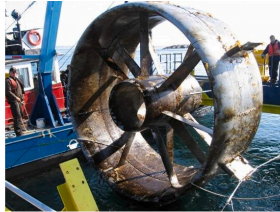
(b) Fouling after six months of the NOVA Innovation turbine (64) (Clean Current Tidal Power Demonstration Project).
