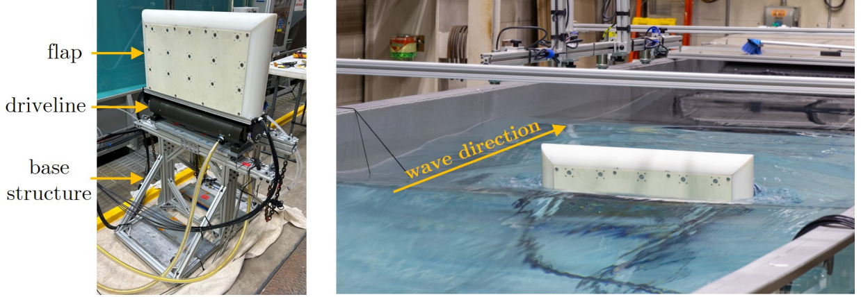
Figure 3.2: [Left] Laboratory-scale OSWEC including flap, driveline, and base structure. The flap is hinged at the driveline, such that it oscillates in response to incident waves or motor torque. [Right] OSWEC operating in SWEL wave tank at the National Renewable Energy Laboratory in Boulder, CO. The flap is surface piercing and waves propagate from bottom left to top right.
