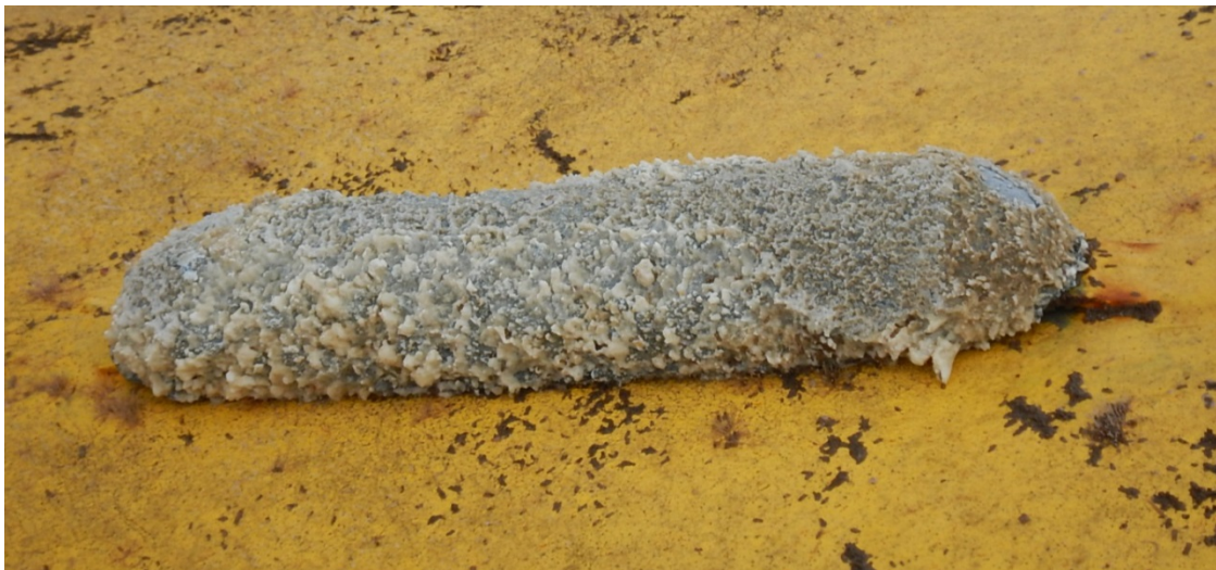
Figure 19 - Turbine Anode (before cleaning)
