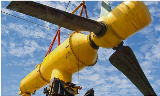
(a) The 500KW DEEPGEN III being lifted.
