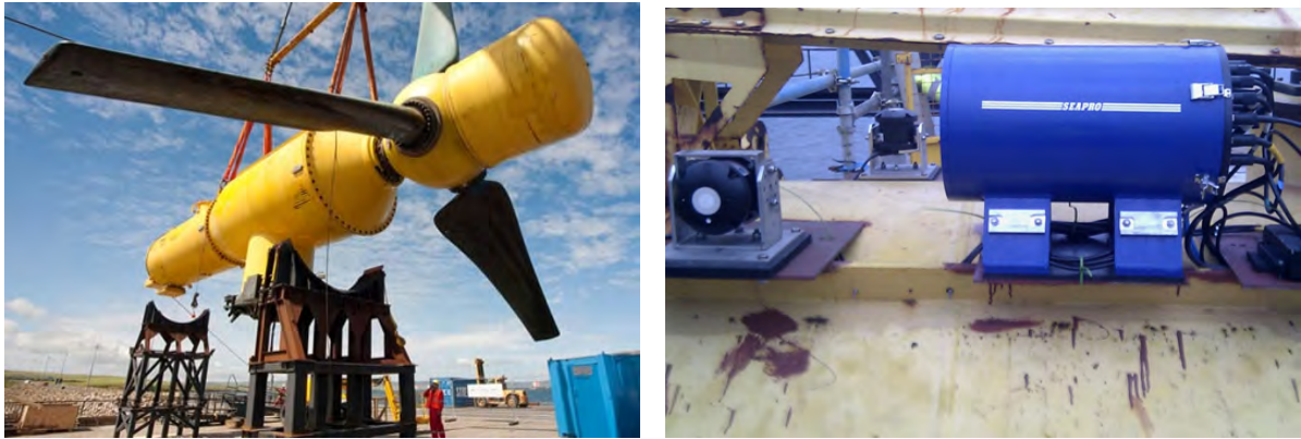
(a) The 500KW turbine on site at Hatston Quay, Orkney, (b) Instrumentation and instrumentation control-box installed on the 500KW machine
